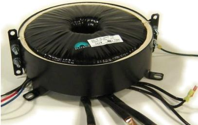
Transformer used in Bryston units, pictured at left, features triple-screens for ultimate noise rejection. Also note metal mounting band that "suspends" the transformer inside the cabinet, further reducing mechanical noise.
