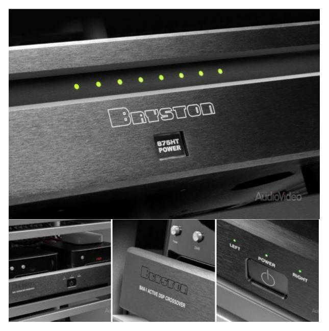
But further in our system - the most interesting. The fact is that the three-way Bryston Mini T speakers that we are going to listen to do not have built-in crossovers. They are designed for separate amplification of bands with active filters in the preliminary path. For this purpose, the **BAX-1** programmable digital crossover was created. The signal coming from the pre-amplifier is first
