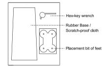
Rubber Base is applicable to CMA400i and Rx200. Rubber Base size: 200\*97\*56mm
