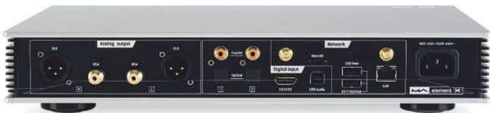
ABOVE: Digital ins include wired/wireless Ethernet and I 2 S on an HDMI socket (up to 768kHz PCM, DSD256 as DoP and DSD1024 natively), USB-B (also 768kHz PCM and DSD256 as DoP), 2x optical/coax S/PDIF and external les via MicroSD and USB-A. Analogue outs (xed or variable) are offered on RCA s and balanced XLRs
