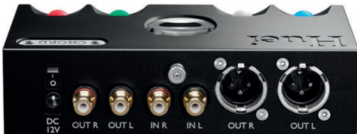
► The Huei is built to the same basic form factor as the company's Qutest DAC. It's a small rectangular box with the distinctive scalloped insets with combination controls and indicators that Chord has been using since the Hugo. The box itself is too small for a power supply, so is fed by a plug-top unit.
