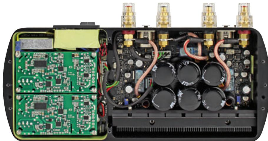
*A lot has been crammed into the Étude – possible through extensive use of surface-mounted components on boards of robotic manufacture. In the left section of the case are switched-mode power supplies. The two power amplifiers occupy the larger remaining section. Eight power MOSFETs – four per channel – can be seen sandwiched against the heatsink (bottom of the picture).*
