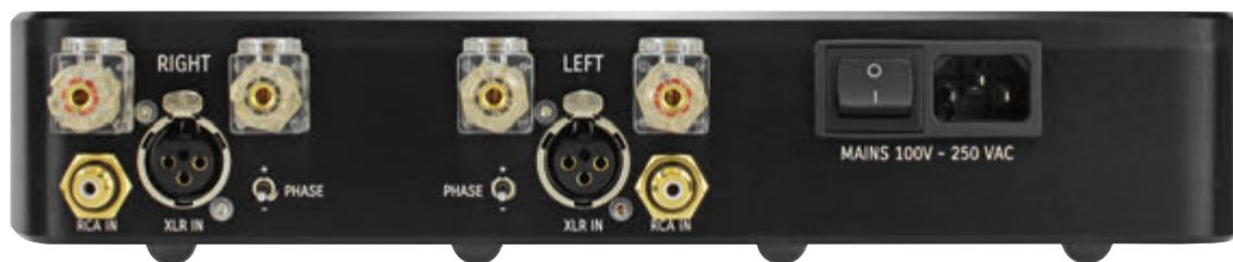
The Étude's rear panel has both balanced (XLR) and unbalanced (phono) inputs. Only one can be used at a time as no switching is provided. Note also the chunky WBT speaker terminals, and the polarity-invert switches that enable the two amplifier channels to be bridged, converting the Étude into a claimed 300-Watt mono powerhouse.
