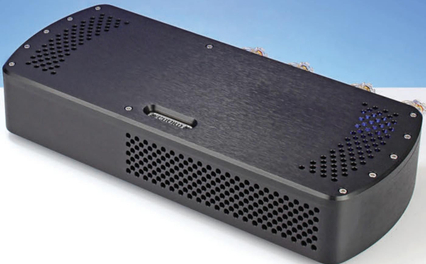
parallel (four devices per channel). Their individual operating conditions are constantly optimised by Franks' dual-feedforward circuitry to ensure that they behave linearly, thereby assuring distortion as low as 0.05% at full power, claimed to be 150 Watts
