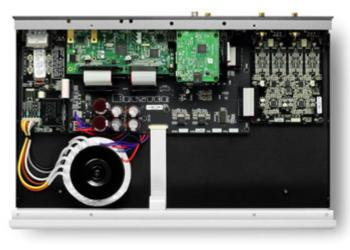
Bryston BDA-3.14 is a streaming player that was created by connecting the BDA-3 digital-to-analog converter with a network module based on the Raspberry Pi platform, previously used in BDP-Pi transport. Both sections are connected by the I<sup>2</sup>S bus, which - as we read on the manufacturer's website - is currently the most accurate method of sending a digital signal.
