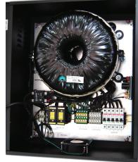
Internal View of Bryston Power Unit: (BIT WMA 100 BAL) A massive toroidal isolation transformer provides complete isolation and ensures sufficient reserve power capabilities to
