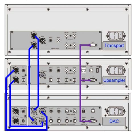
Figure 6 - Mosaic Control remote control connections
