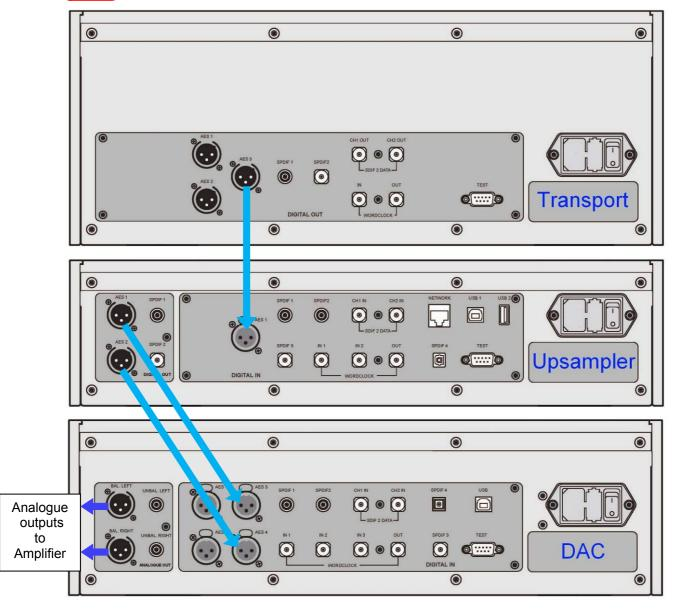
Figure 1 – Connecting the Dual AES output
