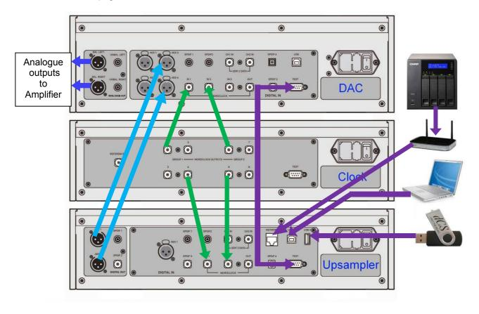
Figure 8 – Using a Vivaldi Upsampler and DAC with a Clock
