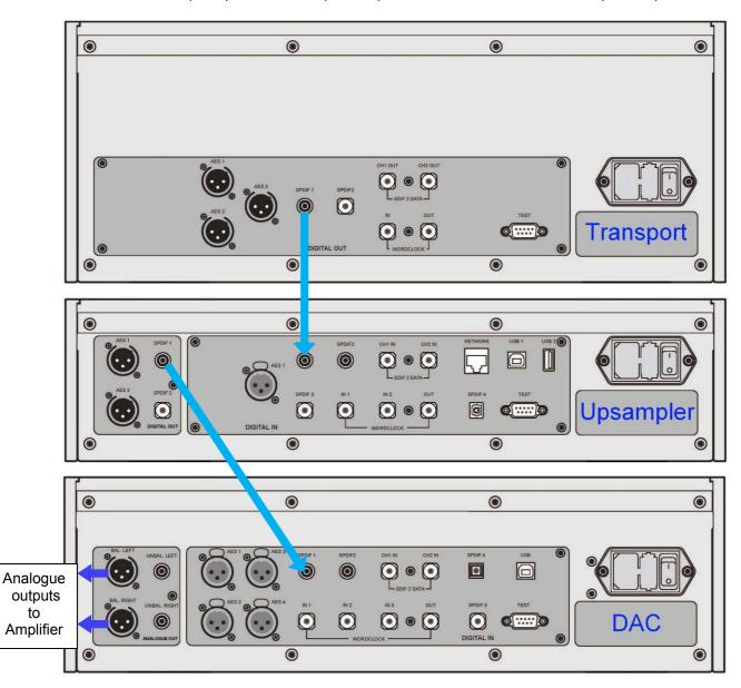
Figure 2 – Connecting a single-wire SPDIF output
