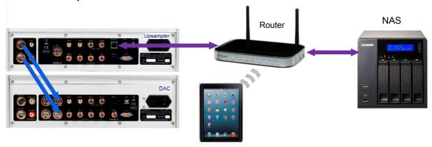
Figure 5 – Using a Vivaldi Upsampler and DAC with a NAS
